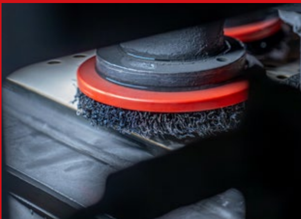
Deburring disc of the SYNTHETIC EDITION on the planetary head of a wet deburring machine
