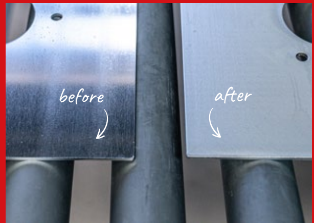
Rounded edges and a matte surface finish in a single operation.
